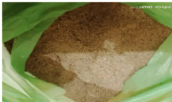
Plate 2: Ground and sieved Banana Stalk
