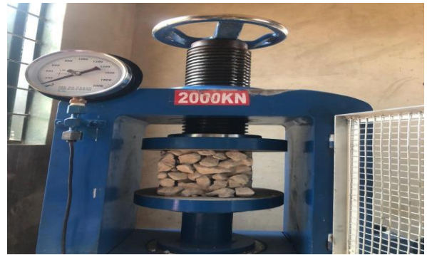
Figure 2: Compressive strength test of pervious concretes
