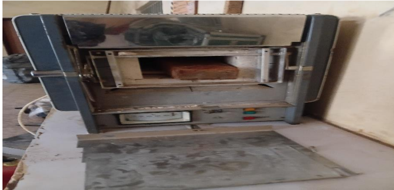
Plate 3: Bricks in the furnace during burning
