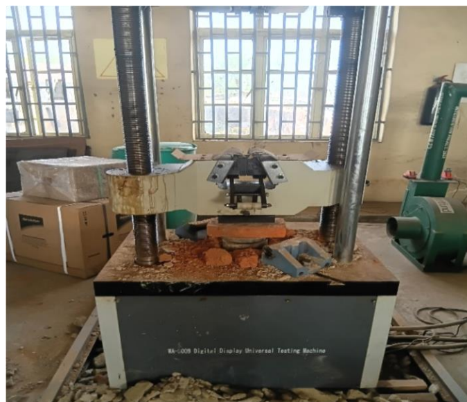
Plate 4: Brick during crushing for compressive strength
