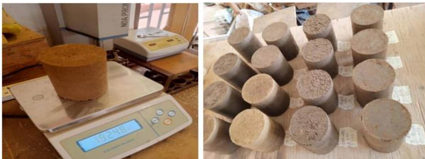
Figure 3: Arranged cylindrical specimen for the Volumetric Shrinkage Strain test.
