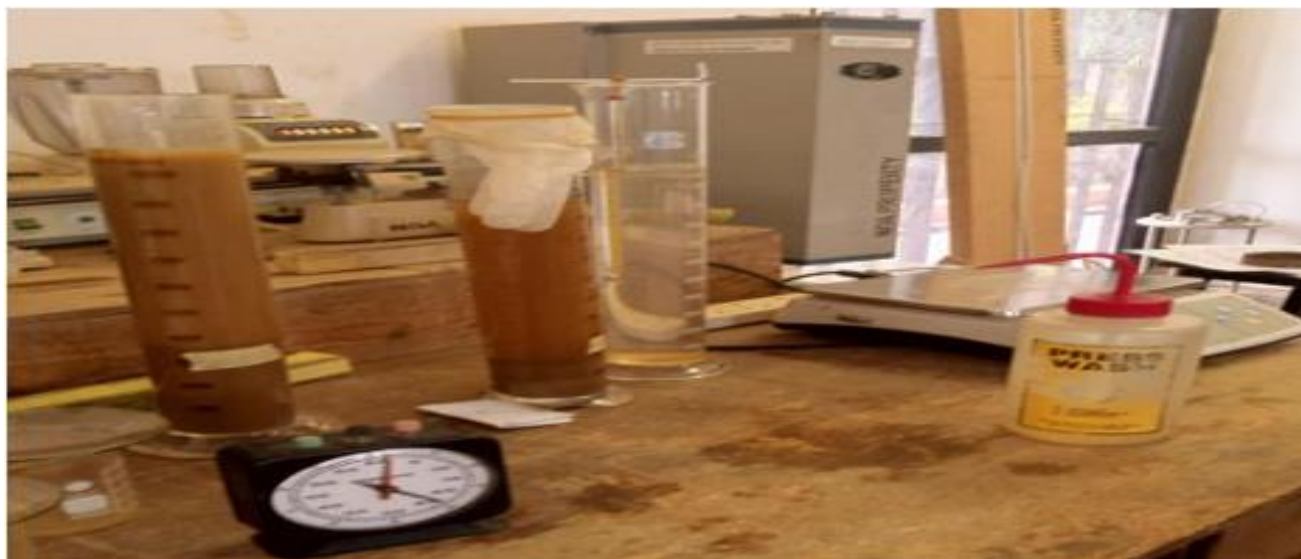
Figure 5: Hydrometer Test of Soil Samples.
