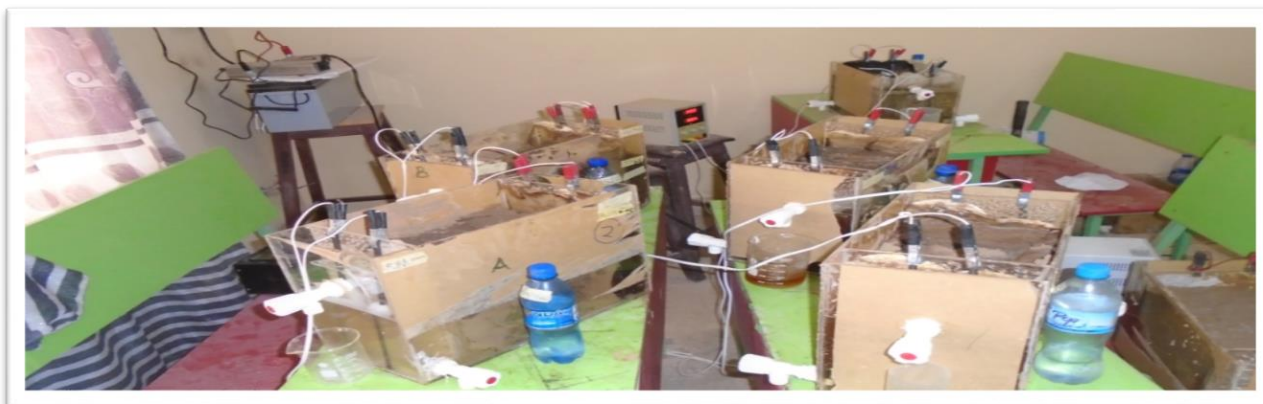
Figure 1: Electrokinetic cell set up for the crude oil contaminated soil.
