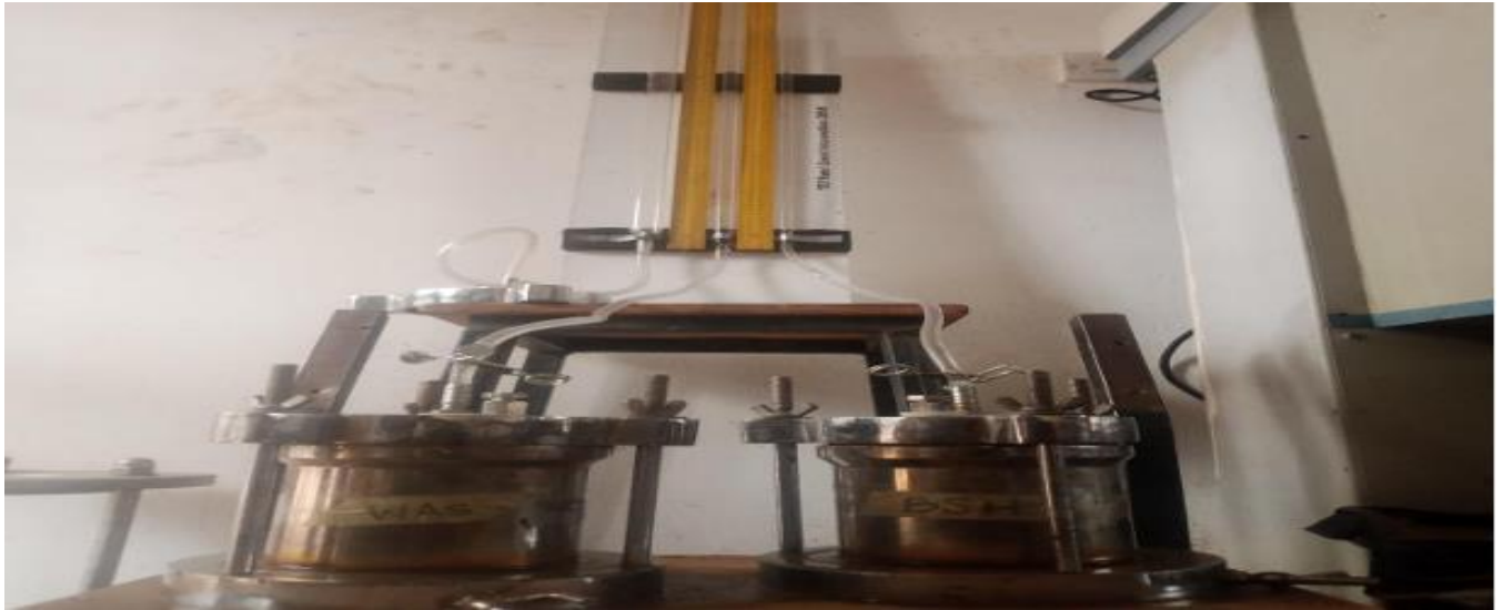
Figure 2: Falling Head Permeameter Set up.
