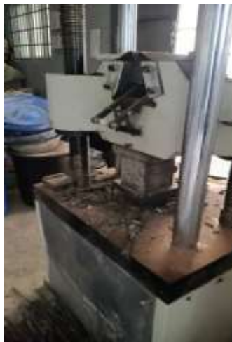
Figure 6: Cube Compressive test
