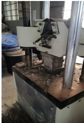
Figure 6: Cube Compressive test
