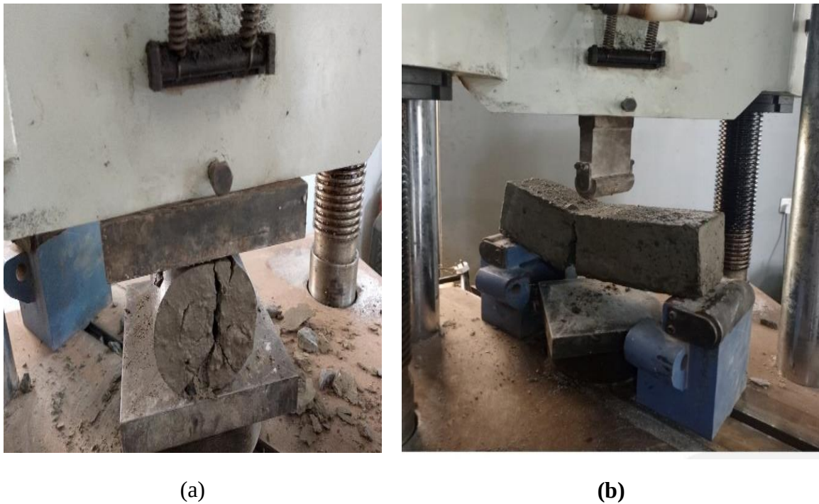
Figure 1 (a & b): Split tensile strength and flexural strength tests
