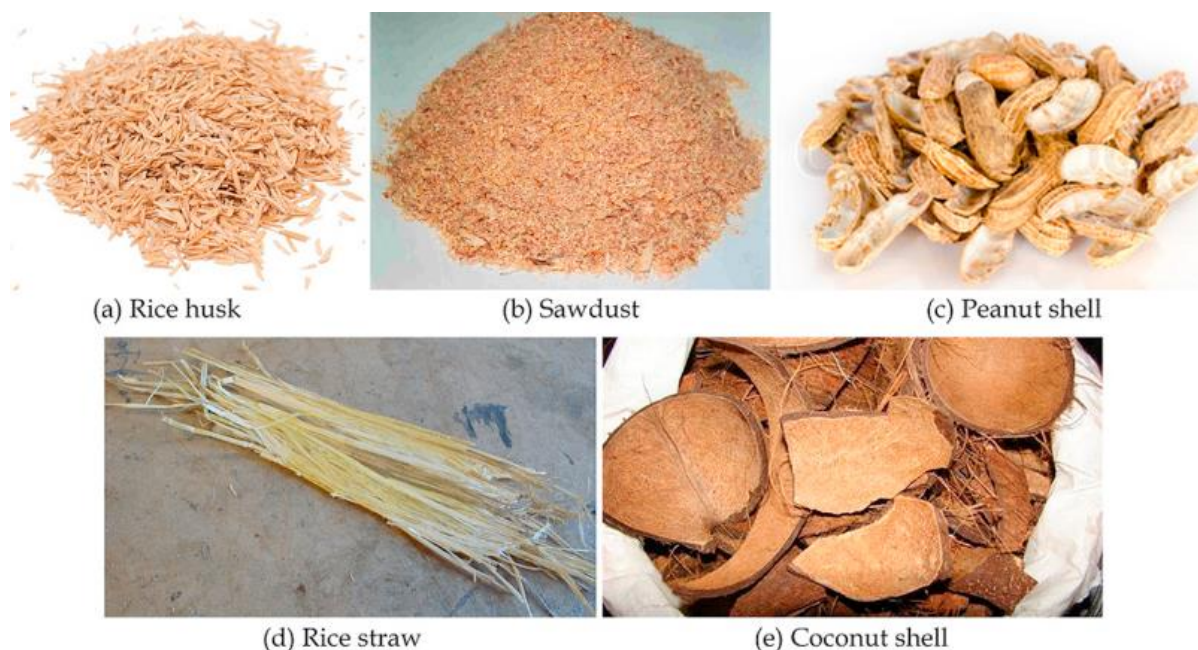
Figure 1: Morphological overview of selected raw agricultural waste materials evaluated for lightweight concrete applications: (a) rice husk (b) wood sawdust (c) peanut (groundnut) shells (d) rice straw and (e) coconut shells. SCM components (a, b) require thermal calcination to optimize amorphous silica content prior to matrix incorporation, whereas macro-elements (c, e) undergo mechanical crushing to serve as alternative aggregates. (Shafigh et al., 2014).
