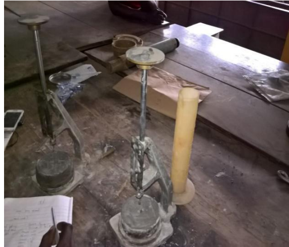
Plate 2: Setting time test.
