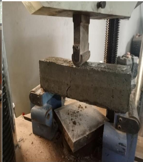
Figure 4: Flexural Test of Concrete
