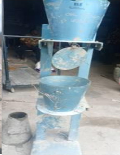
Figure 2: Compaction Factor Test
