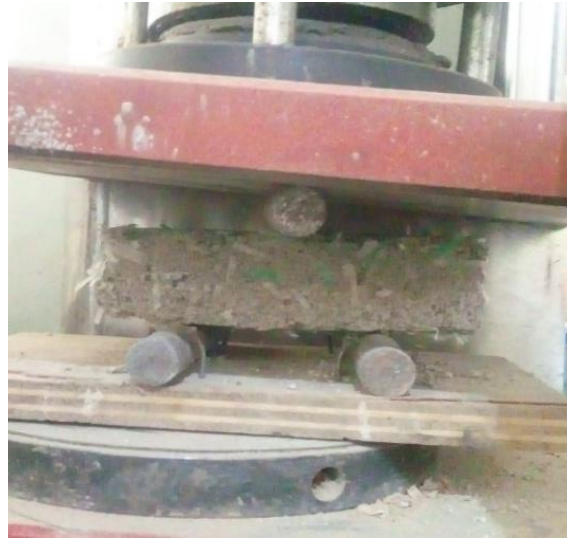
Plate 7: Flexural Test on Fibre Beam
