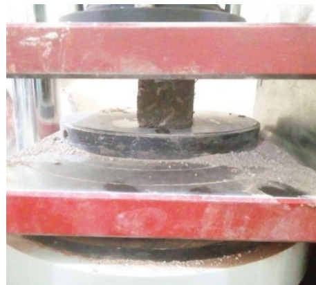
Plate 6: Compressive Test on Cube
