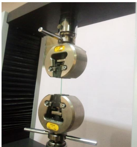
Plate 2: Tensile Test on PP Fibre
