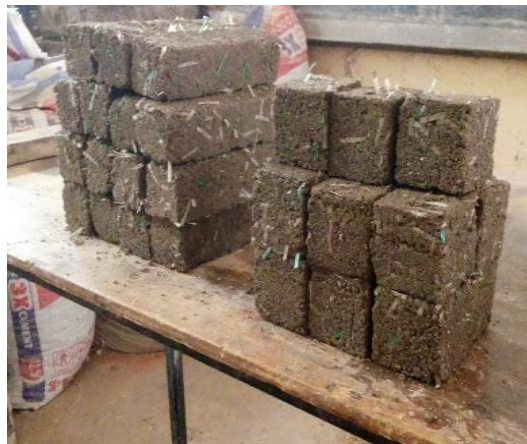
Plate 5: 0.1% PP fibred beams and cubes
