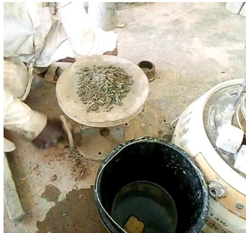
Plate 4: Dropping PP fibred mix
