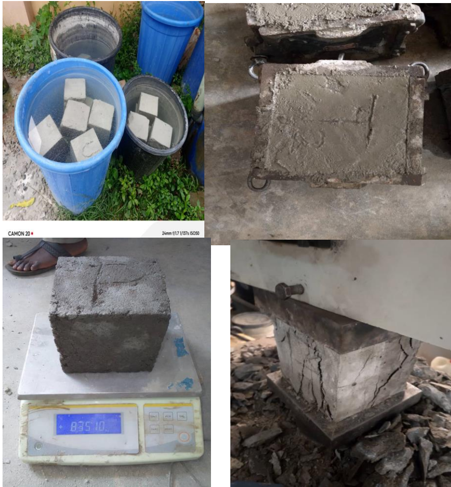
Figure 6: Curing, water immersion Figure 7: Concrete in Metal Mould Figure 8: Weighing Concrete Figure 9: Compressive test.
