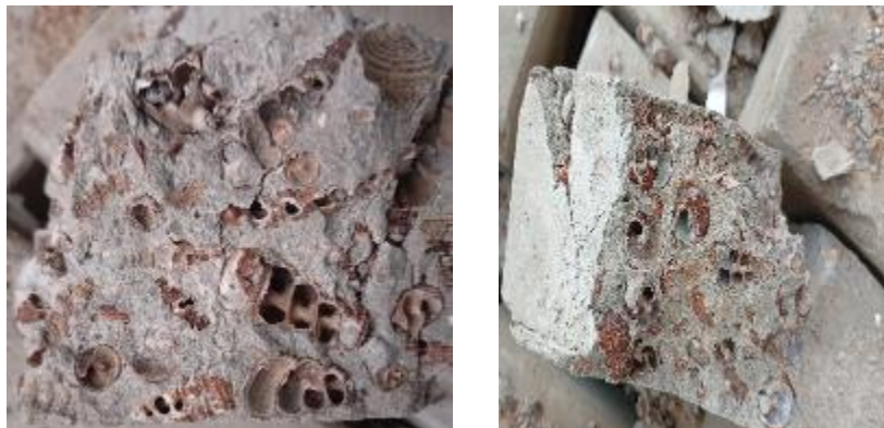
Figure 7: Bonding of PWS and PKS with mortar
