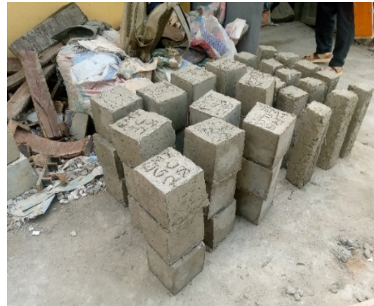
Plate 2: Curing of Concrete samples.
