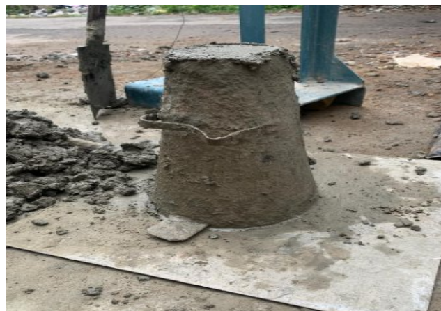
Plate 3: Slump Test of concrete samples
