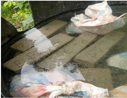
Plate 2: Curing of Concrete samples.
