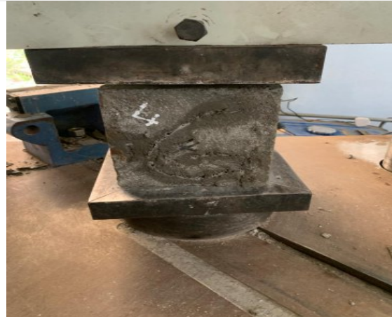
Plate 3: Compressive Test of Concrete samples.
