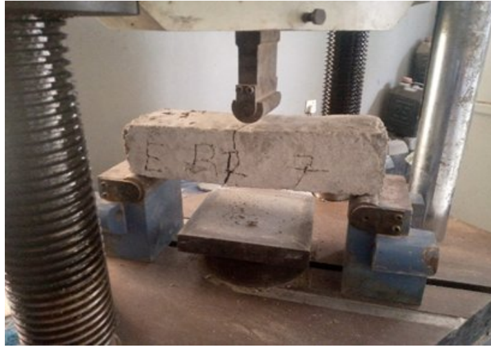
Plate 4: Flexural Test of Concrete samples.
