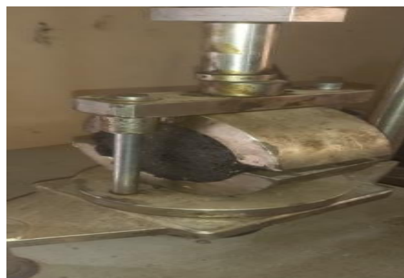
Plate 8: Marshall Stability Test of Samples.
