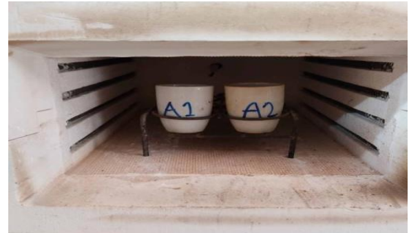
Plate 7: Samples Placed in Furnace.
