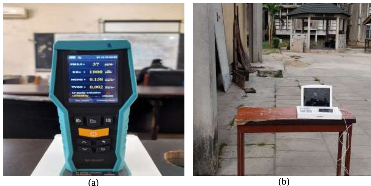
Figure 3: Pictures of the air quality monitors used for this study; (a) Portable Hand-held Br-smart air quality monitor, for indoor air recording; (b) Inkbird air quality monitor for outdoor air recording.
